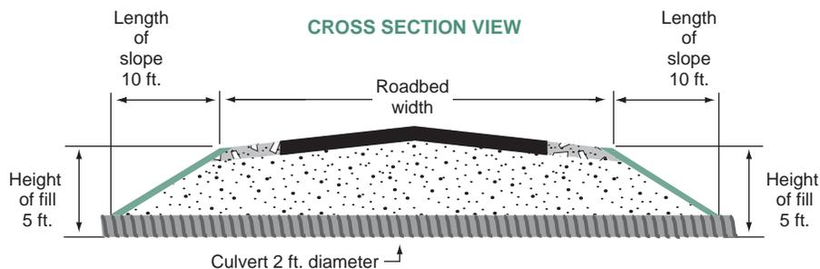
*The length of culvert equals the length of slope on the left and right, plus the roadbed width.*
