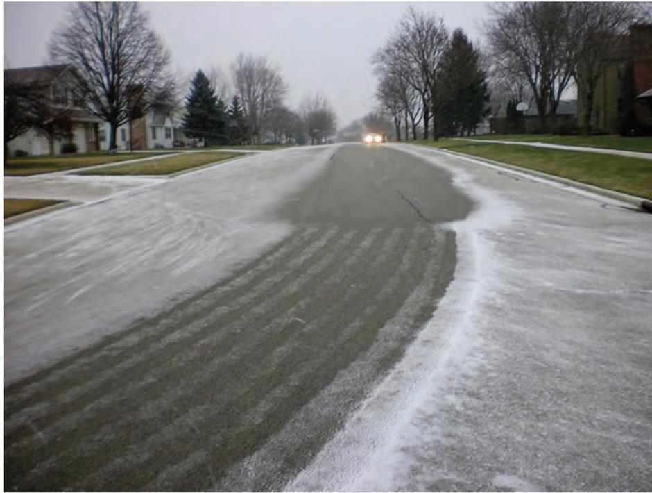
*A test street in De Pere during a snow event illustrates the impact of an anti-icing operation. Treated pavement resists initial snow and ice accumulation prior to plowing.*
